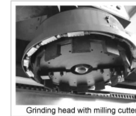
Grinding head with milling cutter
