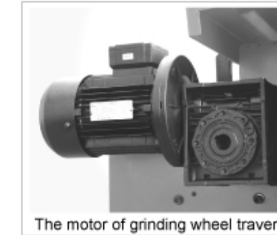
The motor of grinding wheel traverse
